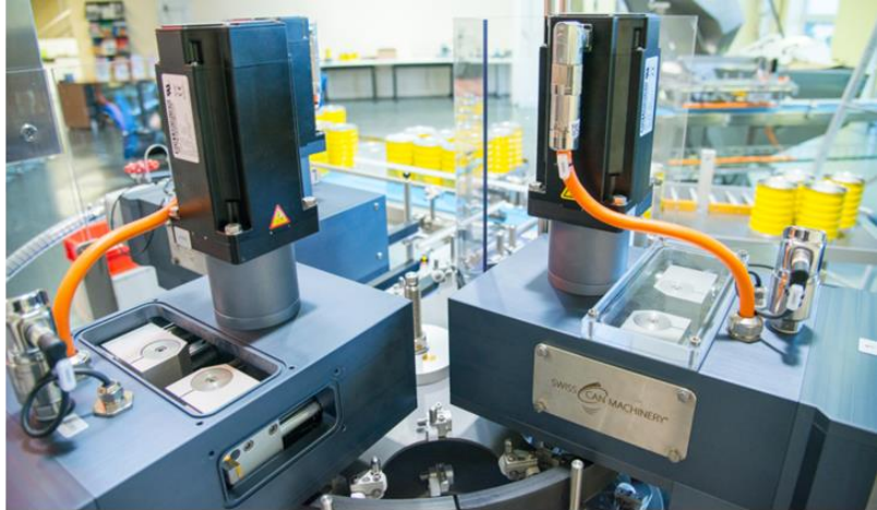
The Swiss company uses standard servo motors from the AKM ranges in areas where hygiene is not relevant.
